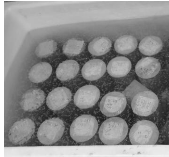
Fig. 4 Concrete samples during curing
